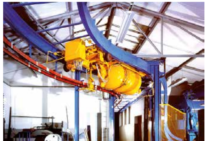
Feed and control of a concrete skipper
