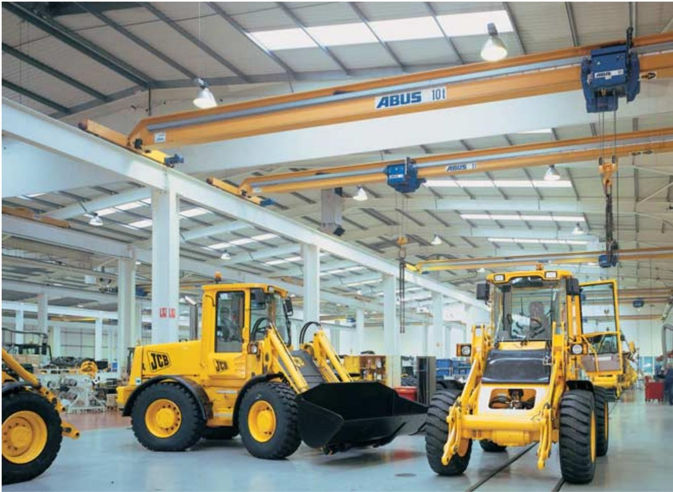
ABUS single girder travelling cranes allow efficient material handling with load capacities up to 16 t and spans up to 39 m even in halls with low ceilings. With a minimal safety clearance between top of crane and factory roof, and the compact dimensions of ABUS crane girders, it is possible to make full use of the available height and to reduce the cost of a new building.
